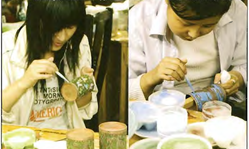
Eyedroppers fill the cloisons with enamel paste before firing in an electric kiln. Heat vitrifies the enamel which settles into the cloisons. Three or four coats of enamel in a variety of colours are applied and fired until the cloisons are completely full.
