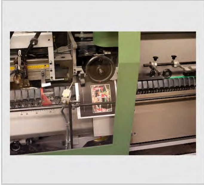
The Cover is applied to the Magazine
