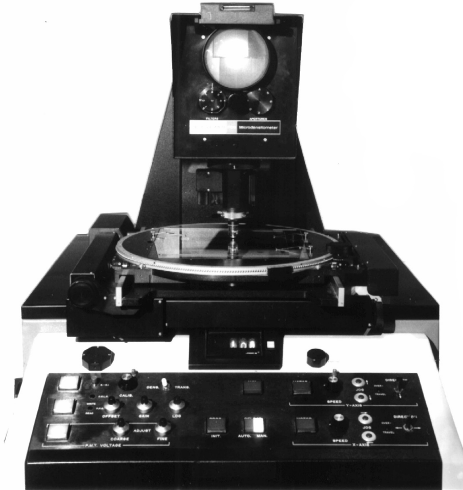
The PDS 1010 microdensitometer. (Flatbed scan of a silver halide monochrome print on an Epson Perfection 4870.)
