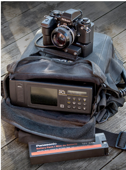
Kodak DCS-100, based on the Nikon F3 camera with a retro-fitted Kodak KAF-100 1.3MB sensor, with its portable Digital Storage Unit (1991). Credit: Marc Aubry (@maoby / Flickr)
