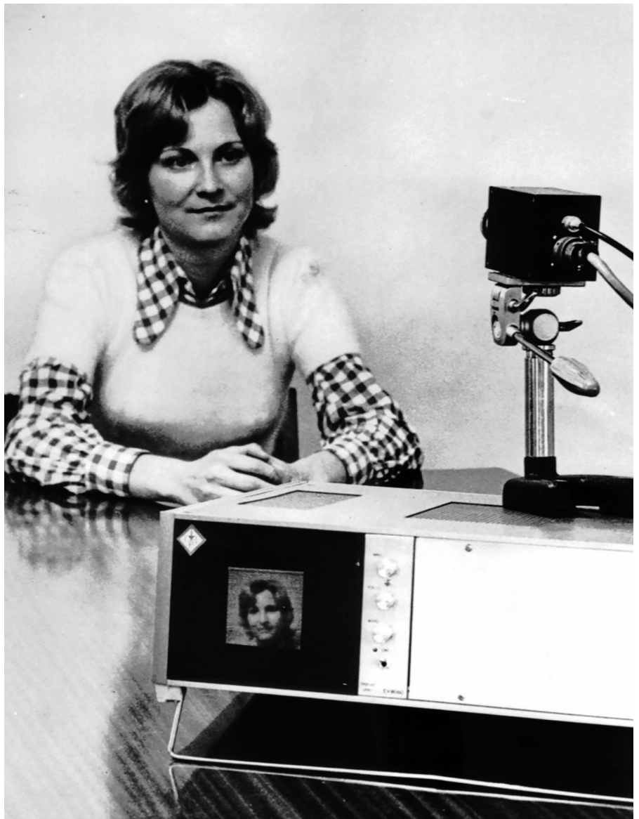
Peter Noble's equipment enabled, for the first time, the capture of a digital photograph from life (1967). Credit: Plessey Research
